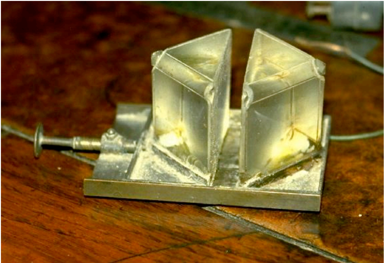
Figure 14. One of Bose's original double-prism attenuators, with adjustable air gap.
