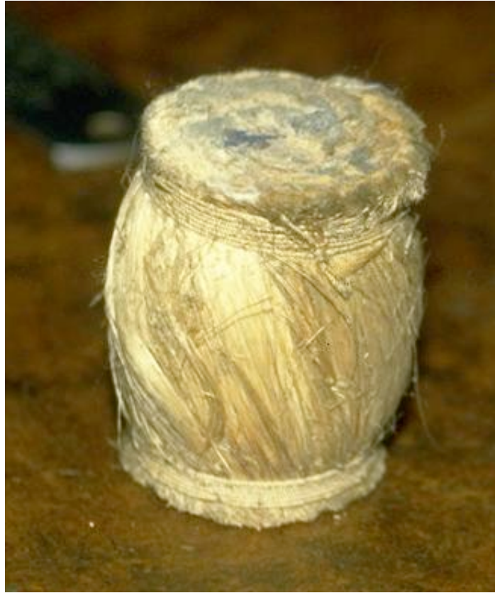
Figure 12. One of the twisted-jute polarizers used by Bose.
