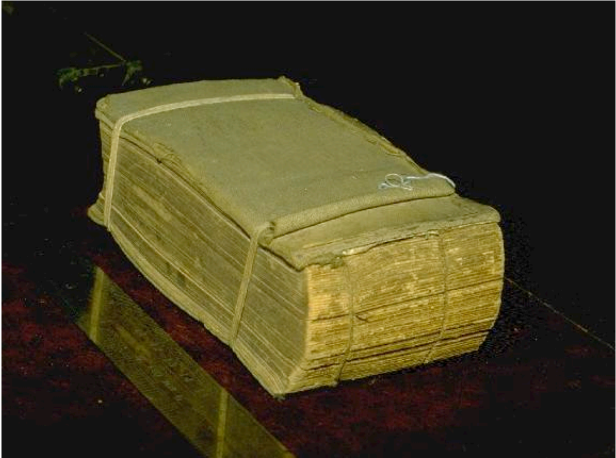
Figure 10. One of Bose's polarizers was a cut-off metal plate grating, consisting of a book (Bradshaw's Railway Timetable) with sheets of tinfoil interleaved in the pages.
